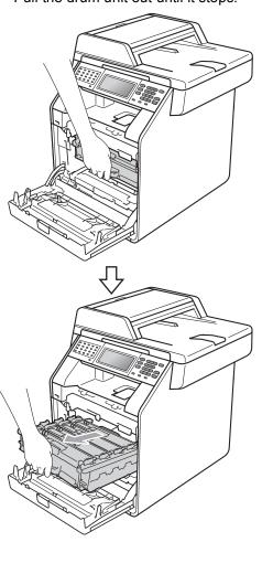
4 Turn the green lock lever (1) at the left of the machine counterclockwise to the release position. Holding the green handles of the drum unit, lift the front of the drum unit and remove it from the machine.
